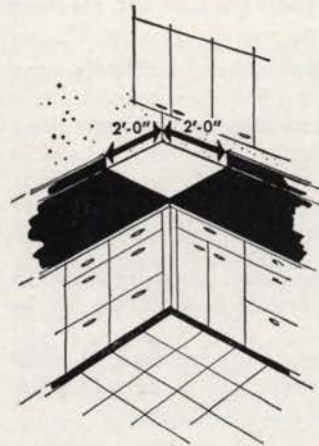
Four feet of wall space is unavailable when a kitchen assembly turns a corner.
